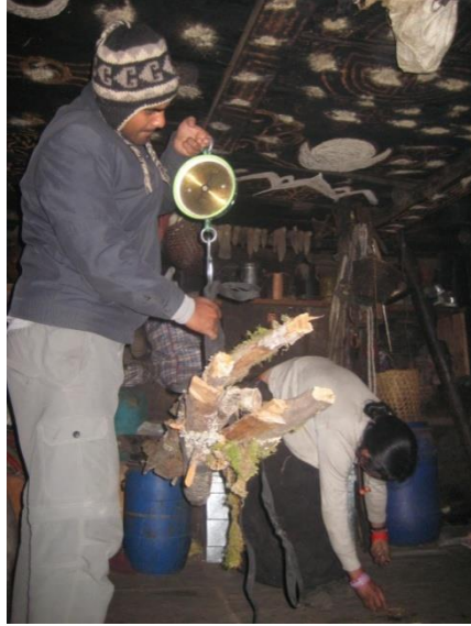
Picture: Researcher weighing fuelwood for fuelwood comparison between TCS and ICS users
