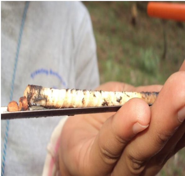
core immediately taken out from a tree
